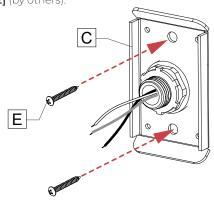
Make electrical connections between the fixture cable [F] and the main power [G] using wire nuts [H] (by others).
