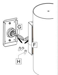
Push all the wires and connectors inside the housing assembly [B].
