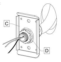
Attach the direct feed bracket **[C]** to the wall with screws [E] (by others).
