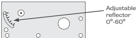
The Asymmetric Projecting Optic cartridges can be rotated upwards on site by 60° to increase vertical projection. Click-stop of 5° intervals, as well as visible aiming marks, provide 13 discrete aiming angles and simplify consistent orientation in long coves.
