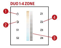
(1) Power: Use this button to turn ON or OFF the fixture Use the color/brightness toggle button to chose between color/brightness. when Blue: brightness is selected, when (2) Brightness/CCT: Yellow: color is selected. (3) Slider: Depending on the mode chosen in 2, the slider will allow the
