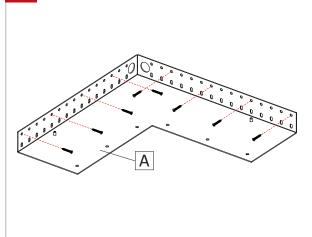
Separate the corner sheet-metal plates (A) from the corner welded extrusion (B) by removing the screws (#6 flat-head screws).
