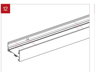
Drill hole (D0.250") in the housing (I) refering to the studs (A) position. Drill another hole (D0.630") for the power cables to be pass thought refering to the shop drawings provided.
