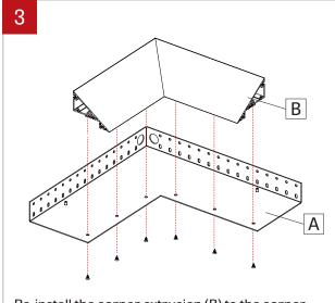
Re-install the corner extrusion (B) to the corner sheet-metal plates (A).
