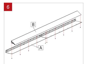
Place the extrusion (B) on top of the sheet-metal plates (A) and secure it with screws.
