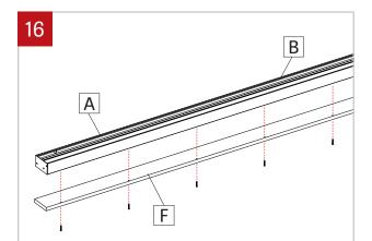
Cut drywall piece (F) according to the dimensions of the ALCOVE kit (7 3/8" recommanded width). Mark a line on the drywall piece of 15/16" from the edge and then place it under the metal plates. Screw it to the extrusion (B) (#6 Drywall screws 1.0" long, supplied by other) using the line as guide.
