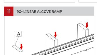
Find the placement of the studs and mark on the fixture where the first stud (A) is, then place a mark at every 16" on the fixture.
