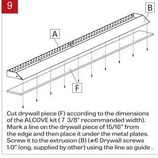
the aligners (C) as guide. Secure the extrusions (B)
