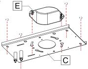
Drill holes (1/4" diameter) following the marks drawn from previous step 2. Install #8 screws anchors [G].
