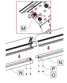
Note: Reflector must be reinstalled with the screw and plastic washer that was originally supplied. If not, it can result in an electrical failure.
