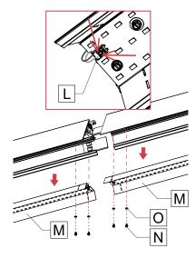
Note: Reflector must be reinstalled with the screw and plastic washer that was originally supplied. If not, it can result in an electrical failure.
