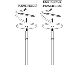
In the case where an <u>emergency circuit</u> is required, the wires to the emergency circuit will be passed through a second stem.
