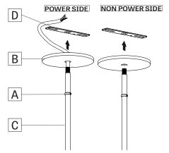
Make sure that the power to the fixture is turned off. Slide the slip ring (A) and the canopy (B) onto the stem (C) and leave some space. Screw the junction box crossbar (D) onto the stem (C).
