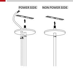
In the case where the luminaire is installed on a **grid ceiling**, the power cable will pass outside of the stem.
