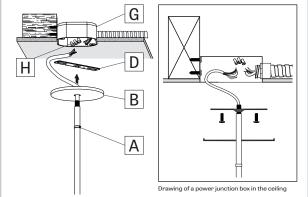
Raise the fixture and tighten the junction box crossbar (D) with screws (by others) to the junction box (G). Make wire connection with wire connectors (H). Then slide the canopy (B) and thighten the set up with the slip ring (A).
