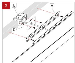
Screw back the junction cover (C) on the junction box (E) and then screw the wall bracket (A) to the wall using anchors.
