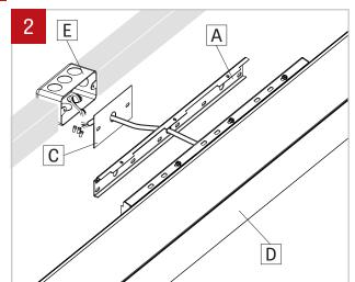
Pass the electrical wires throught the wall bracket (A) and junction cover (C) and make electrical connection between fixture (D) and junction box (E).
