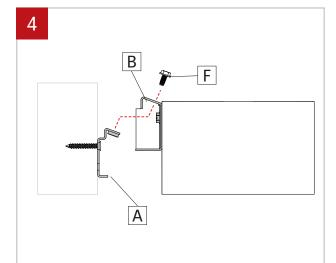
Insert fixture bracket (B) into wall bracket (A) and secure in place with supplied screws (F). Do not overtighten.
