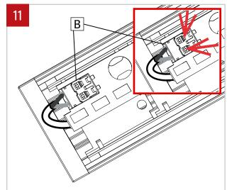
Disconnect LED molex connector (B) by taking a pointed object and pressing on the two tabs on the top.
