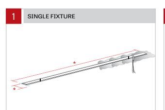
Prepare the area where the fixture is going to be installed. Cut hole in the drywall according to the dimensions [\*] in the client drawings.
