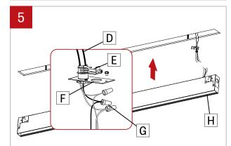
Install power cable (D) (by other) through the BX connector (E) (by other) and install onto the power plate (F) provided. Make electrical connections between power cable (D) and fixture cables using electrical marettes (G). Reinstall the power plate [G] to the fixture (H). Number of wires may vary.
