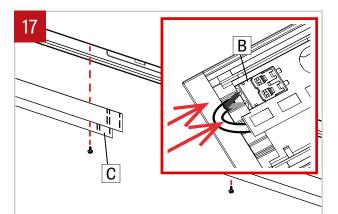
Reinstall the cartridge (C) and reconnect the LED molex connector (B). **NOTE: connect blue wire into the negative (-) terminal and the red wire into (+) positive terminal.** Make sure that the wires are not hiding any LED diode. Screw the cartridge back in place by using screw with plastic washer. Do not apply too much pressure.
