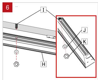
Insert the fixture (H) into pre-cut hole in drywall, aligning threaded rods (I) with holes in top of fixture (H). Put washers (J) and tighten nuts (K) to secure the fixture (H).
