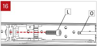
Remove the screw (L) on the joiner and put it in a
