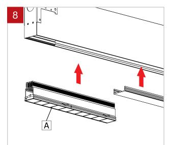
Reinstall the extrusion clusters (A) and the lens or blank.
