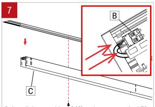
Reinstall the cartridge(s) (C) and reconnect the LED molex connector (B). NOTE: connect blue wire into the negative (-) terminal and the red wire into (+) positive terminal. Make sure that the wires are not hiding any LED diode. Screw the cartridge back in place by using screw with plastic washer. Do not apply too much pressure.
