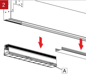
Remove clusters (A) and/or remove the lens or blank by using
