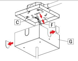
Make the connection between the fixture quick connector (F) and the main power quick connector (C). Punch out the knock outs of the canopy (G) to allow the canopy to fit over the conduits.
