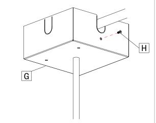
Secure the canopy (G) by tightening the pan head screw (H).
