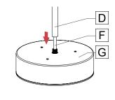
Adjust the cable length by cutting and stripping the fixture cable [F] to the desired length for the height of the fixture. Remove any excess cable length.
