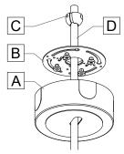
Adjust the stem **[D]** to the desired length for the height of the fixture. Position the swivel ball **[C]** at the level of desired stem length. Lock the swivel ball using the set screws **[E]**.
