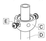
Drill a hole through both sides of stem [D]. Cut off the excess stem length (above the swivel ball [C]).
