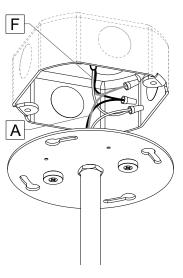
Mount and turn the mounting plate [D] to place on the junction box [G]. Tighten screws to secure the mounting plate [D] to the junction box.
