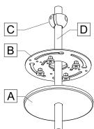
Adjust the stem **[D]** to the desired length for the height of the fixture. Position the swivel ball **[C]** at the level of desired stem length. Lock the swivel ball using the set screws **[E]**.
