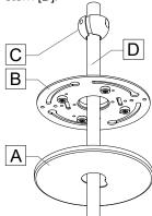
Adjust the stem [D] to the desired length for the height of the fixture. Position the swivel ball [C] at the level of desired stem length. Lock the swivel ball using the set screws [E].
