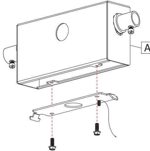
Install the Custom Junction Box (A) onto the Ceiling with the Conduit.
