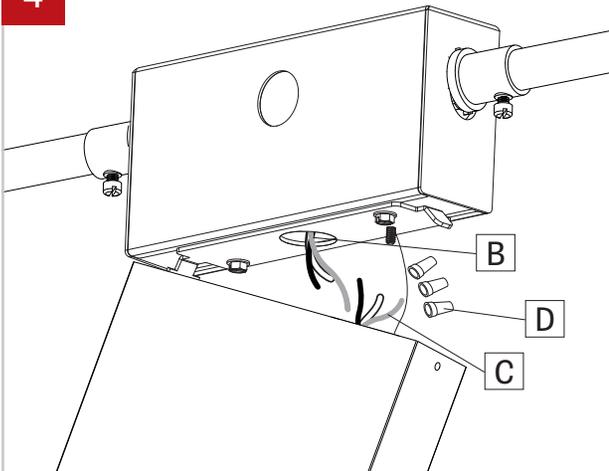
Make the Connections between the Main power cables (B) and the Fixture Cables (C) using Marettes (D)
