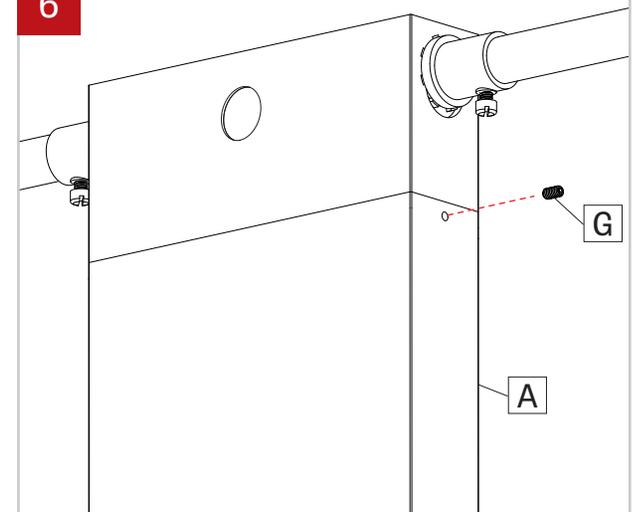
Secure the Fixture (A) by installing the Set screw (G) onto the fixture.
