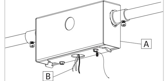
Pull out the Main power cables (B) out of the Junction box (A).
