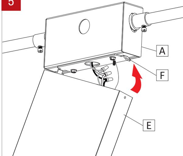
Install the Fixture (E) onto the Junction box (A) by hooking onto the brackets (F).
