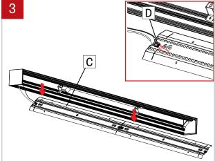
Disconnect LED molex connector (D) by taking a pointed object and pressing on the two tabs on the top. Remove the cartridge (C) and keep it in a safe place.
