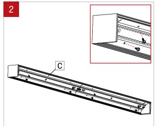
Unscrew the cartridge (C) and keep the screws in a safe place.
