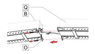
4 INSTALL THE FIXTURE TO THE CEILING.
