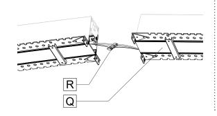
Join the fixture [B] to the fixture [Q]. Attach the two fixtures by fastening screws on the joiners [O].
