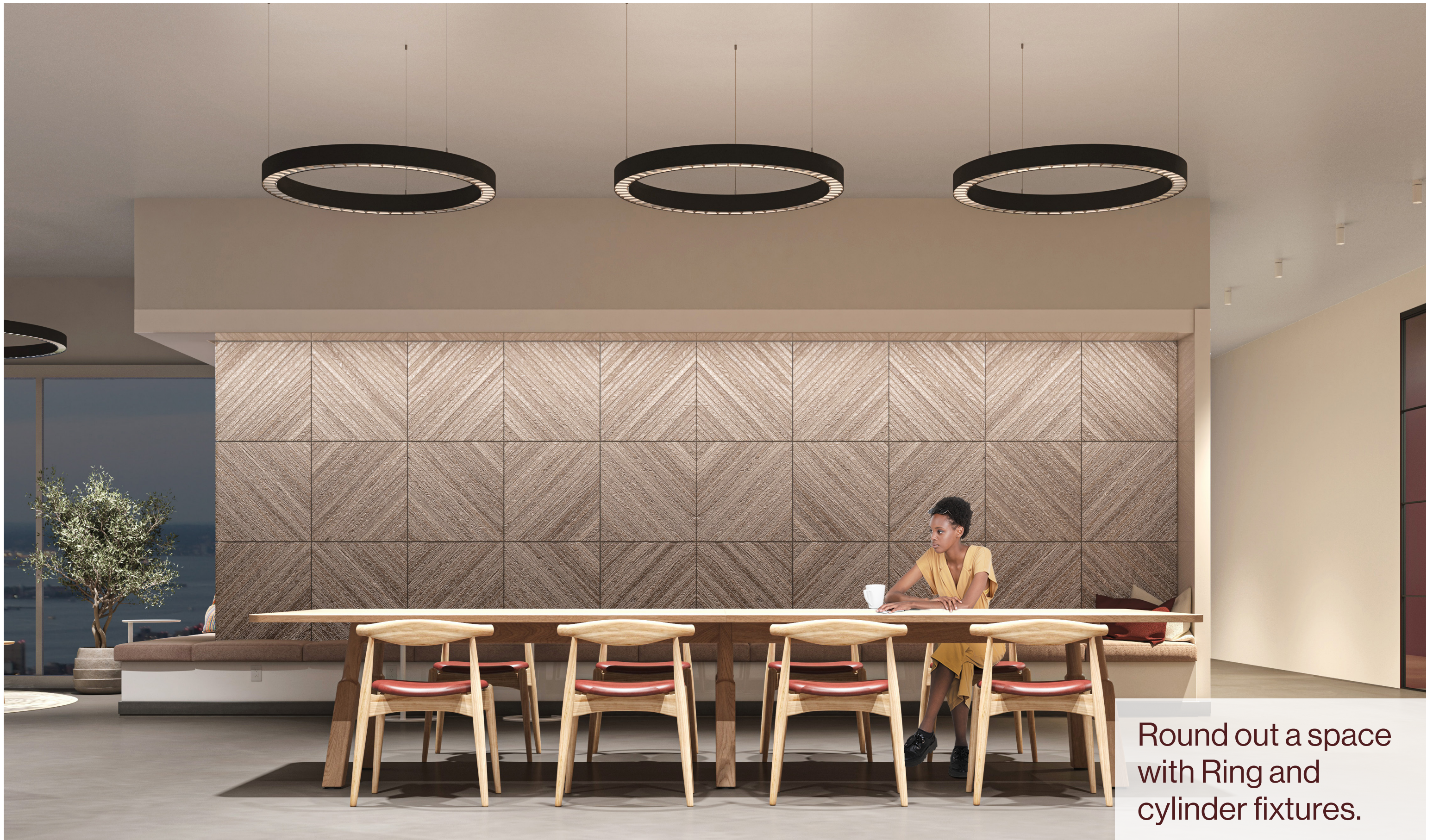
Curvia 2 Prism Ring direct/indirect (3' diameter) pendants with DPO™. Background: Via 3 Perimeter. Right: Pivot mono point cylinders.
