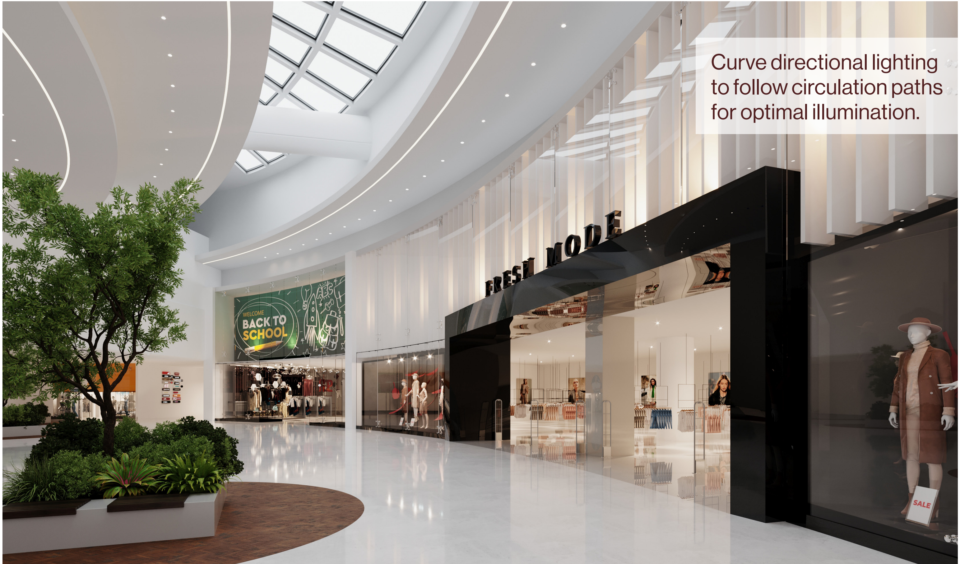
Showcasing Curvia 4" with 4" Voila downlights using 50-degree beams.
