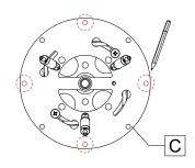
Remove the mounting plate. Drill holes (1/4" diameter) following the red marks. Install #8 screw anchors [E].
