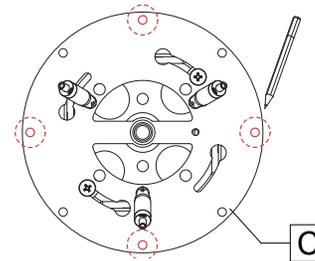
Remove the mounting plate. Drill holes (1/4" diameter) following the red marks. Install #8 screw anchors [E].
