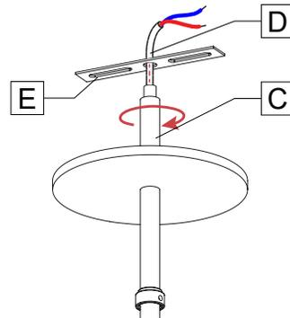
Screw the stem [C] on the fixture [F].
