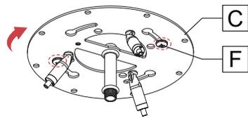
Use #8 screws [G] to fasten the mounting plate [C] to the ceiling.
