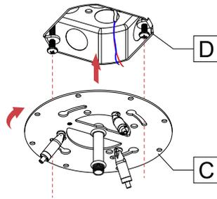
Use the mounting plate [C] as a model to mark 4 holes.
