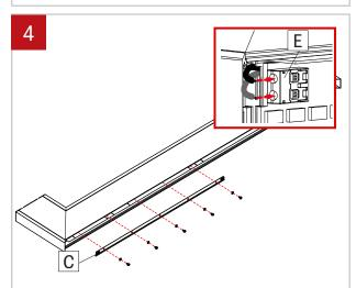
Replace LED boards (C) and screw back in place the first one by using screws with washers. Do not apply too much pressure. Reconnect LED molex connector (B) to the first board.
