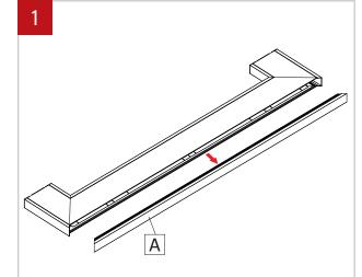
Make sure the power to the fixure is turned off. Remove the lens (A) from the fixture.
