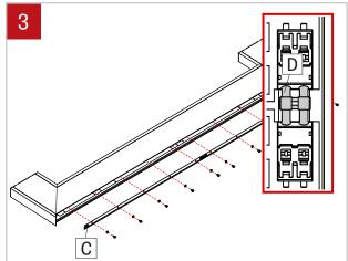
Unscrew the LED boards (C) directly from the fixture and remove them. If need to remove just one board, disconnect the coupler (D) between the two boards connectors after having unscrew the LED board (C).
