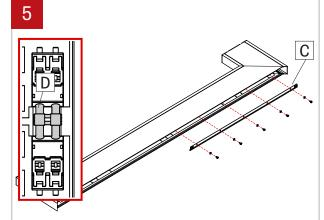
Insert coupler (D) into connector of the first board. Insert coupler (D) into connector of the second board. Screw second LED board (C) to the fixture by using screws with plastic washers. Do not apply too much pressure. Make sure that the coupler stays in place in between the two boards.
