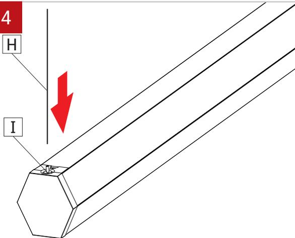
Insert the aircraft cable (H) into the cable gripper (I). Adjust the cable (H) length (cut it if needed). Secure the cable gripper (I) by tightening the safety nut on the gripper.
