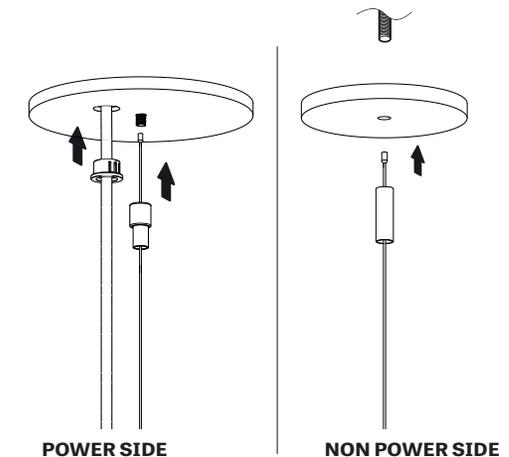
For a continuous system, repeat steps 1 to 3 for all mounting and 4-5 for the first fixture in the run.
