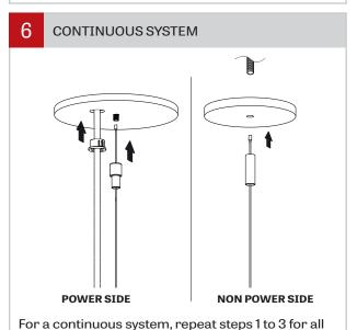
mounting and 4-5 for the first fixture in the run.
