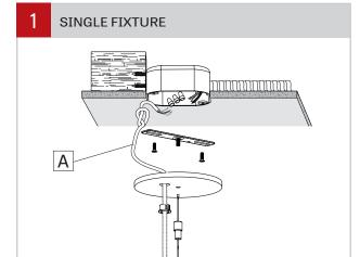
Locate ceiling mounting points according to supplied client drawing. Make a knot in the power cord (A) and then connect it to the ceiling power feed.
