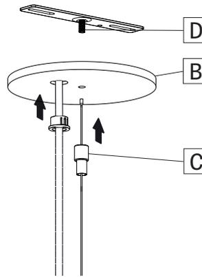
Secure canopy (B) with slip ring (C) on threaded rod (D).
