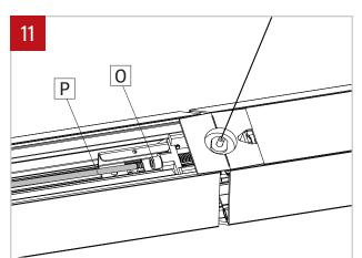
Put back in place the provided screw (0) (using 3/16" Ball-End Screwdriver (P) provided). Make sure that no wires are placed in between the extrusions, preventing the fixtures to be joined. Tighten the screw (O) to pull the extrusions together. Repeat steps 6 to 11 for all others fixtures in the run.
