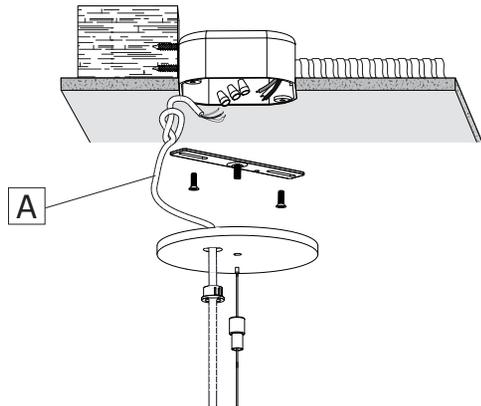
Locate ceiling mounting points according to supplied client drawing. Make a knot in the power cord (A) and then connect it to the ceiling power feed.
