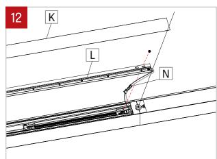
Replace the cartridges (L) by reconnecting the quick connector (N). Make sure that the wires are not hiding any LED diodes. Screw the cartridge (L) back in place. Put the top lens (K) back in place.
