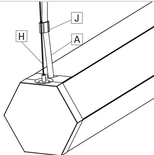
Secure power cord (A) to aircraft cable (H) with plastic clip (J).
