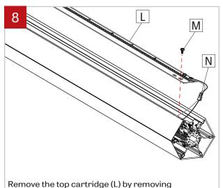
the screws (M). Disconnect the cartridge by disconnecting the quick connector (N). Keep the
