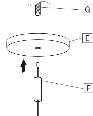
Secure canopy (E) with cable coupler (F) on crimp strut (1/4"-20) (G) (by other).
