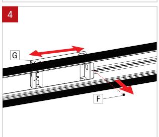
Remove the driver box screw (F) and keep it in a safe place. Slide the driver box (G) to be able to fit it between wall studs.
