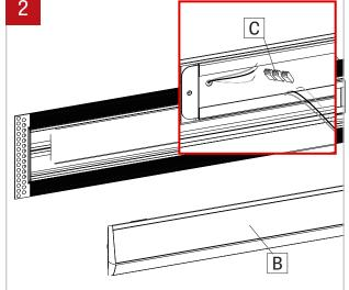
Remove the optic (B) and disconnect the quick connectors (C). Place the cartridge in a safe place.
