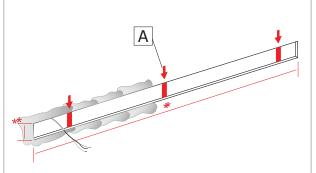
Make the hole in the wall with the right dimension (\*) using provided client drawing. Be sure to have access to the main power cable. Mark on the wall where the studs (A) are.
