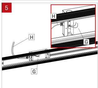
Pass the main power cable (H) through the driver box (G) without doing the connection.
