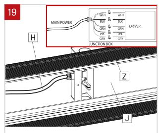
Make the electrical connection between the main power (H) and the driver (J) with wire nut (Z) (provided by others). Number of wires may vary.
