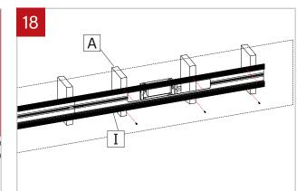
Drill hole (D0.250") on the mud flanges (I) refering to the studs (A) position. Make sure they are aligned (using the alignment pins already in the alignment holes). Screw the fixture in place (screws not provided) to the wall.
