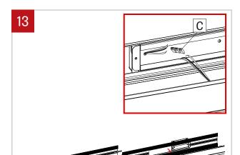
Remove the optic (B) from the second fixture and disconnect the quick connectors (C). Place the cartridge in a safe place.
