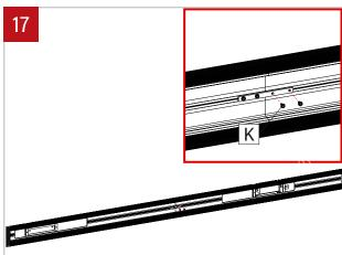
Insert the housing in the hole, slide it against the first section so there is no gap between the 2 adjacent sections. Attach the 2 housings together using the 2 joining screws (K) previously removed from the joining bracket.
