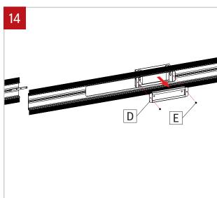
Remove the driver box cover (D) by unscrewing it.
