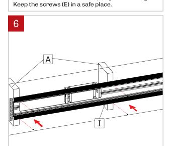
Drill hole (D0.250") in the housing (I) refering to the studs (A) position. Screw the fixture in place (screws not provided) to the wall.
