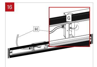
Pass the main power cable (H) through the driver box (G) without doing the connection.
