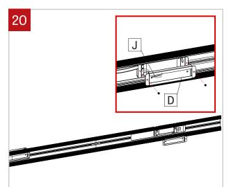
Reinstall the driver box cover (D) in place. Make sure to pass the wires (J) from the driver through the holes.
