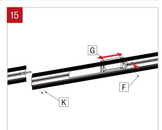
Remove the joining screws (K) and keep it in a safe place. Remove the driver box screw (F) and keep it in a safe place. Slide the driver box (G) to be able to fit it between wall studs.
