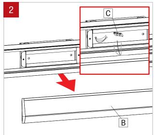
Remove the optic (B) and disconnect the quick connectors (C). Place the optic (B) in a safe place.
