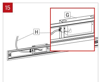
Pass the main power cable (H) through the driver box (G) without doing the connection.
