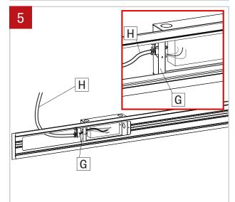
Pass the main power cable (H) through the driver box (G) without doing the connection.
