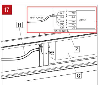
Make the electrical connection between the main power (H) and the driver (G) with wire nut (Z) (provided by others). Number of wires may vary.
