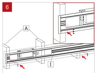
Drill hole (D0.250") in the housing (I) refering to the studs (A) position. Screw the fixture in place (screws not provided) to the wall.
