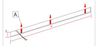
Make the hole in the wall with the right dimension (\*) using provided client drawing. Be sure to have access to the main power cable. Mark on the fixture where the first stud (A) is, then place a mark at every 16" on the fixture.
