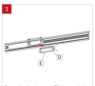
Remove the driver box cover (D) by unscrewing it. Keep the screws (E) in a safe place.
