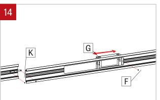
Remove the joining bracket (K) and keep it in a safe place. Remove the driver box screw (F) and keep it in a safe place. Slide the driver box (G) to be able to fit it between wall studs that were premarked on the fixture.
