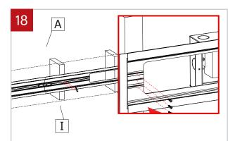
Drill hole (D0.250") on the housing (I) refering to the studs (A) position. Insert the housing in the hole, slide it against the first section so there is no gap between the 2 adjacent sections. Make sure they are aligned (using the alignment pins already in the alignment holes). Screw the fixture in place (screws not provided) to the wall.
