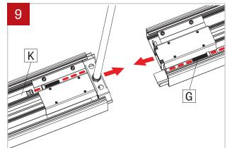
Join fixtures using align pins as guide. Put back in place the provided screw (G) (using 3/16" Ball-End Screwdriver (K) provided). Make sure that no wires are placed in between the extrusions, preventing the fixtures to be joined. Tighten the screw (K) to pull the extrusions together.
