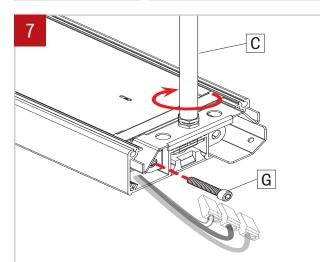
Remove the screws (G) on the joiner and put them in a safe place. Screw the stems (C) onto the end of the fixture. Repeat the stem installation onto the second fixture.
