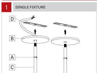
Make sure that the power to the fixture is turned off. Slide the slip ring (A) and the canopy (B) onto the stem (C) and leave some space. Screw the junction box crossbar (D) onto the stem (C).
