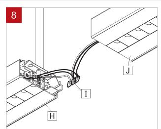
Connect wires between joining fixtures (H) and (J) using wires connectors (I). Push the connectors inside the second fixture (J). Number of wires may vary.
