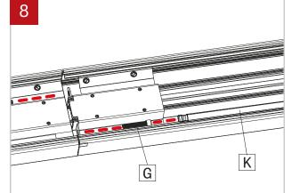
Join fixtures using align pins as guide. Put back in place the provided screw (G) (using 3/16" Ball-End Screwdiriver (K) provided). Make sure that no wires are placed in between the extrusions, preventing the fixtures to be joined. Tighten the screw (K) to pull the extrusions together.
