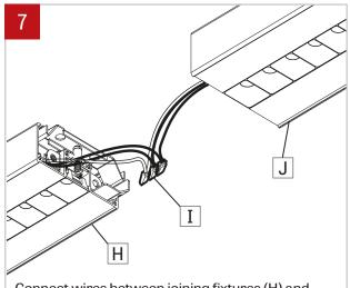
Connect wires between joining fixtures (H) and using wires connectors (I). Push the connectors inside the second fixture (J). **Number of wires may vary.**
