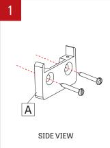
Locate wall bracket position using provided client drawing. Install mounting brackets (A) to wall. Align with structural stud (need double studs – distance between screws is 1.250") or use metal anchors with min. length 1.250". Flat head Philips drive screw, nominal size #10, min. length 1.250".
