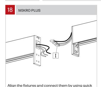
connectors (I). Push the wires inside the second
