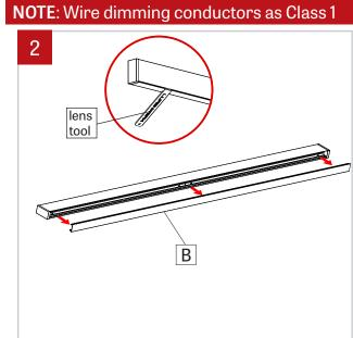
Remove lens (B) with the included lens tool.
