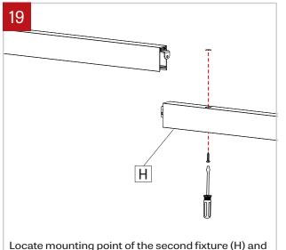
install it. Fasten the second fixture (H) to the wall
