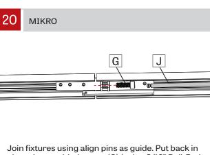
Join fixtures using align pins as guide. Put back in place the provided screw (G) (using 3/16" Ball-End Screwdriver (J) provided). Make sure that no wires are placed in between the extrusions, preventing the fixtures to be joined. Tight the screw (G) to pull the extrusions together. Repeat steps 16, 17, 19 and 20 for all other fixture. Then tighten all screws on mounting brackets.
