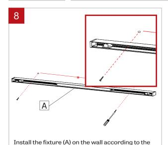
dimensions [\*] given in the client drawings. Screw
