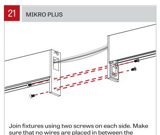
extrusions, preventing the fixtures to be joined.
