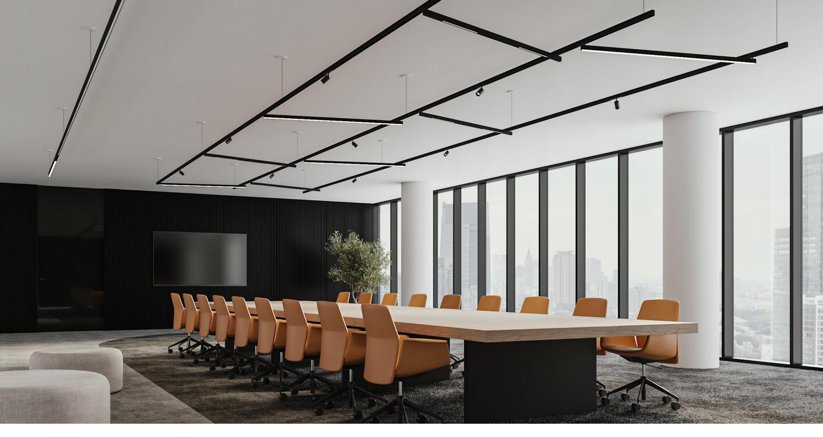
Right: Mini Pivot Dot 1.5" mounted on Mini Pivot Pendant Track with Mini Pivot Prism and HLO mounted on Bridge modules Left: Mini Pivot Linear with Prism, HLO, and Blanks Bridge modules mount across two tracks and tap into the power system to serve as additional tracks.
