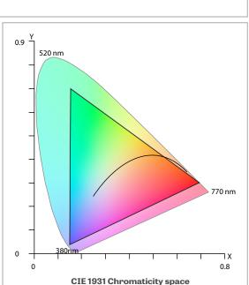
The above diagram overlays the full gamut of colors attainable with the RGBW on top of the CIE 1931 color space. Any color point inside of the triangle can be obtained by setting the correct output levels for each of the individual red, green, blue, and white channels.
