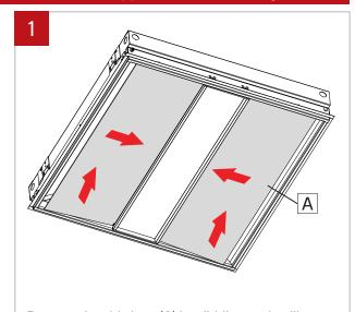
Remove the side lens (A) by slidding and pulling
