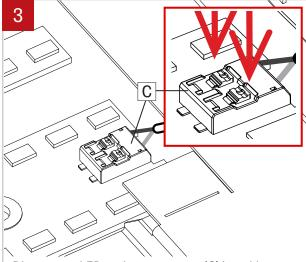
Disconnect LED molex connector (C) by taking a pointed object and pressing on the two tabs on the top. Repeat for second board.
