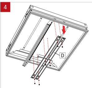
Unscrew LED boards (D) and remove them from the fixture.
