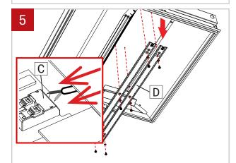
Replace LED boards (D) and reconnect LED connector (C). NOTE: connect white wire into the negative (-) terminal and black wire into (+) positive terminal. Screw the LED boards (D) back in place by using screws with plastic washers. Do not apply too much pressure.
