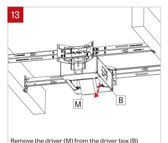
by pushing it to the bottom of the box and then
