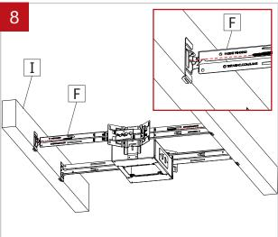
Raise the fixture between the stud and secure
