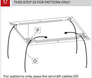
through the cable brackets (P), which are attach to
