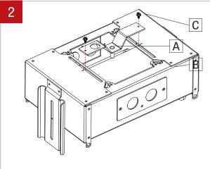
Unscrew and remove the cable coupler bracket (A) from the driver remote box (B). Keep the screws (C) and the bracket (A) in a safe place.
