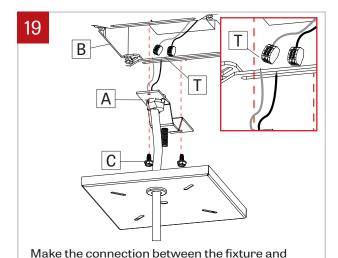
the driver with the quick connector (T). Then, fix the coupler bracket (A) to the driver box (B) with screws (C). Use the marks on the driver box to
