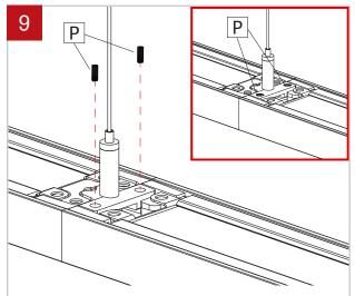
Secure both sides of the joiner (P) with the pre-install set screws. Be sure to tight them <u>flush</u> with the joiner.
