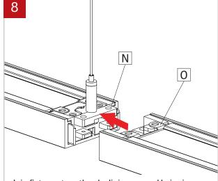
Join fixtures together by lining up and bringing together both the male (N) and female (O) sides of the joiner.
