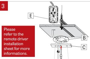
Locate ceiling mounting points according to supplied client drawing. Pass the low voltage power cord through the canopy, make a knot in the power cord (E) and then connect it to the ceiling power feed. Install the cable holder plate (B) and canopy (C). Installation may differ dependind of your type of ceiling, please refer to the remote driver installation sheet for more infos.
