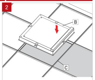
Insert the fixtures (B) above the ceiling grid. Lower fixture (B) onto the t-bar grid (C).
