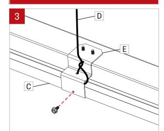
For additional safety, a security wire (D) can be attached from mounting brackets (E) and a screw can be used to fix to the fixture to the T-bar grid (C).
