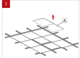
Remove ceilling tiles (A) where the fixture will be installed and adjacent tiles for easy access during installation. NOTE: Once installation is complete, luminaire needs to be accessible from above for visual branch circuit connection inspection.
