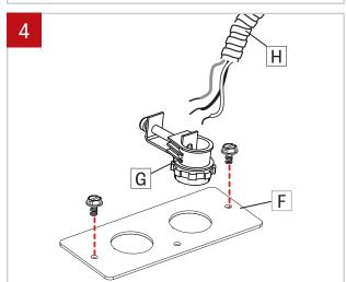
Remove power plate (F) from fixture and install BX connector (G) (by others) and BX cable (H) (by others) through the power plate. Tighten BX connector (G) screw.
