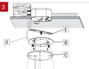
Locate ceiling mounting points according to supplied client drawing. Pass the power cord through the canopy, make a knot in the power cord (X) and then connect it to the ceiling power feed. Install the junction box cross bar (E), cable holder plate (B) and canopy (C).
