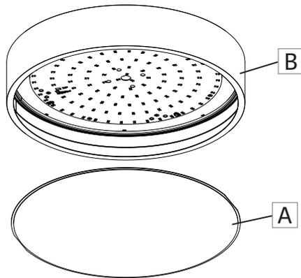
Push the lens (A) up and guide it out of the housing (B).
