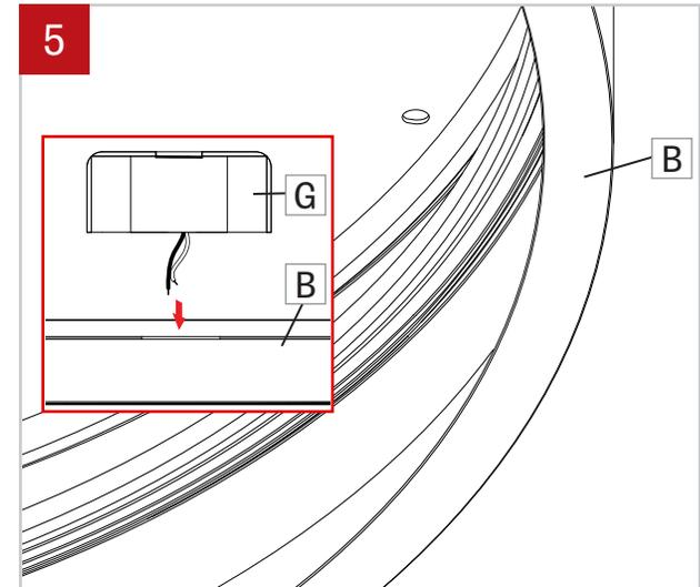
Pass the power wires from the junction box (G) through the hole in the housing (B).
