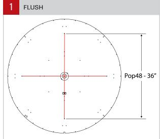
Locate the rod mounting points [\*] in the ceiling according to the client drawings.
