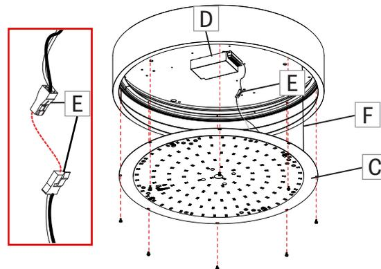
Unscrew the LED plate holder (C) to get access to the driver (D). Disconnect quick connectors (E) between driver and LED board. Remove security cable (F).
