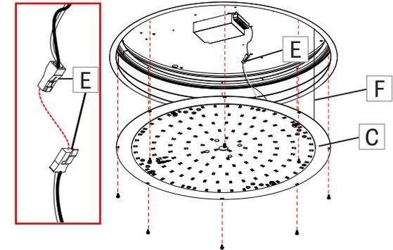
Attach security cable (F). Make wires connection between the driver and the LED board by connecting quick connectors (E). Screw the LED plate holder (C) back in place.
