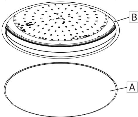
Align and tilt the lens (A) to insert it back into the housing (B).
