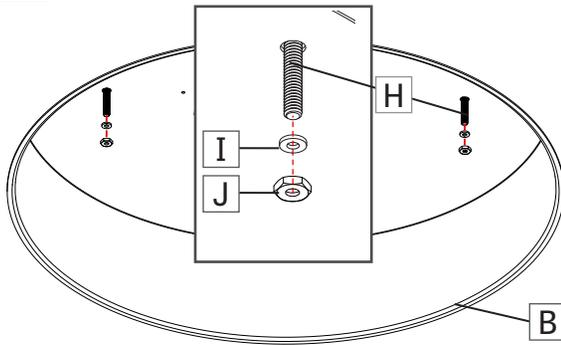
Insert fixture's housing (B) into pre-cut hole in drywall, aligning threaded rods (H) with holes in top of the fixture's housing (B). Put washers (I) and tighten nuts (J) to secure the fixture's housing (B) at an appropriate height.
