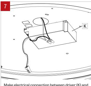
Make electrical connection between driver (K) and power wires from junction box.
