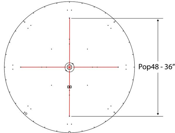
Locate the rod mounting points [\*] in the ceiling according to the client drawings.
