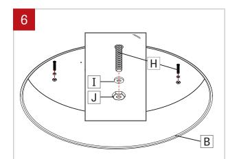
Insert fixture's housing (B) into pre-cut hole in drywall, aligning threaded rods (H) with holes in top of the fixture's housing (B). Put washers (I) and tighten nuts (J) to secure the fixture's housing (B) at an appropriate height.
