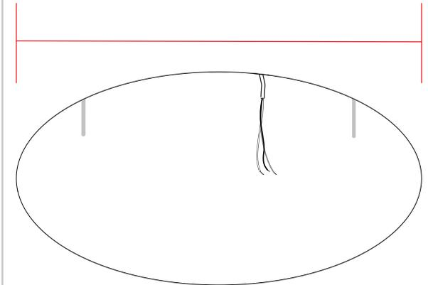
Cut out hole in the drywall according to the dimension [\*] given in the client drawings.
