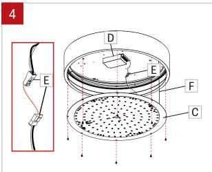
Unscrew the LED plate holder (C) to get acess to the driver (D). Disconnect quick connectors (E) between driver and LED board. Remove security cable (F).
