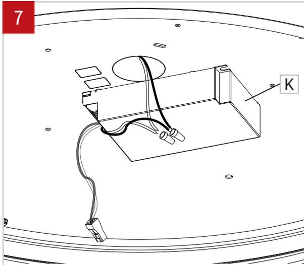
Make electrical connection between driver (K) and power wires from junction box.
