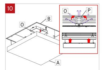
Squeeze, align and insert the springs (0) into the brackets (P) that are further inside the housing. Once all the springs (0) are properly installed, slowly push the diffuser (A) in the housing (B) as far as the brackets (P) allow.
