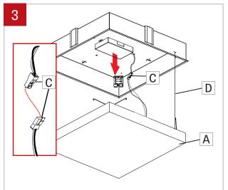
Disconnect quick connectors (C) between driver and diffuser (A). Remove security cable (D).
