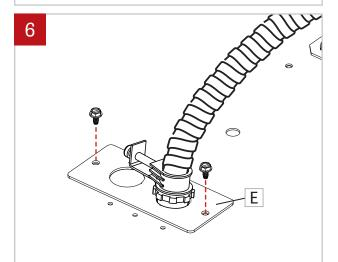
Push connected wires inside the fixture. Reinstall power plate (E) onto fixture by refastening screws to power plate (E) and fixture.
