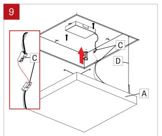
Attach security cable (D). Make the wires connection between the driver wires and the LED board (A) using the quick connectors (C).
