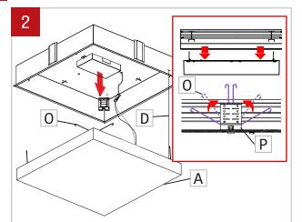
Pull down the diffuser (A) to get acces to the springs (O). Squeeze the springs (O) to release them from the brackets (P). Once all the springs (O) have been released, slowly lower the diffuser (A) retained by security cable (D).
