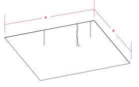
Cut hole in the drywall according to the dimension [\*] given in the client drawings.
