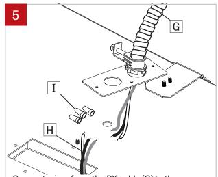
Connect wires from the BX cable (G) to the fixture driver wires (H) using wire nuts (I). Ensure connections comply with local and national electrical codes.
