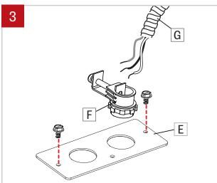
Rotate fixture and remove power plate (E) from fixture. Install BX connector (F) (by other) and BX cable (G) (by other) trought the power plate. Tightened BX connector (F) screw.
