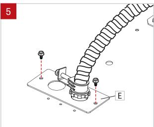
Push connected wires inside the fixture. Reinstall power plate (E) onto fixture by refastening screws to power plate (E) and fixture.
