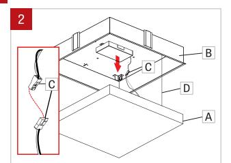
Push slowly the diffuser (A) until it unlocked. Lower the diffuser (A) from the housing (B). Disconnect quick connectors (C) between driver and diffuser (A). Remove security cable (D).
