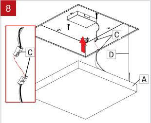
Attach security cable (D). Make the wires connection between the driver wires and the LED board (A) using the quick connectors (C).
