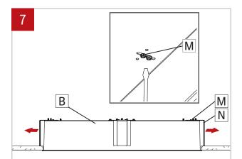
Untighten the screws (M) on the mounting brackets (N) and push the mounting brackets (N) away from housing. When brackets are fully extended, tighten the screws (M) back to secure the housing (B).
