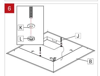
Insert fixture's housing (B) into pre-cut hole in drywall, aligning threaded rods (J) with holes in top of the fixture's housing (B). Put washers (K) and tighten nuts (L) to secure the fixture's housing (B).
