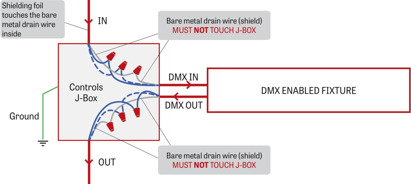
Low capacitance DMX cable to next fixture
