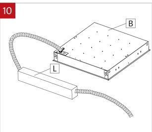
If a remote battery pack (L) was ordered with fixture (B), place Remote battery pack not further than 50 ft from the fixture ( for an 18 gauge wire).
