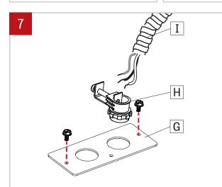
Remove power plate (G) from fixture and install BX connector (H) (by other) and BX cable (I) (by other) trought the power plate. Tightened BX connector (H) screw.
