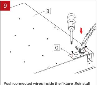
power plate (G) onto fixture (B) by refastening
