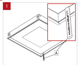
Make sure the power to the fixure is turned off. Place lens tool (A) in between frame and lens, as shown.
