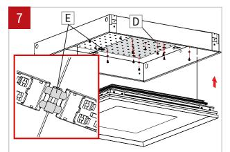
Insert coupler (E) into connector of the first board. Insert coupler (E) into connector of the second board. Screw second LED board (D) to the fixture by usign screws and washers. Do not apply too much pressure. Make sure that the coupler stays in place in between the two boards.
