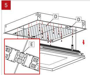
Unscrew LED boards (D) and remove them from the fixture. If need to remove just one board, disconnect the coupler (E) between the two boards connectors after having unscrew the LED board (D).
