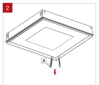
**Slowly** pull down lens frame on four corners using the lens tool (A).
