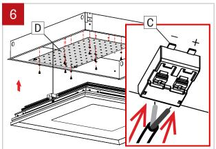
Replace LED boards (D) and screw back in place the first LED board by using screws and plastic washers. Do not apply too much pressure.
