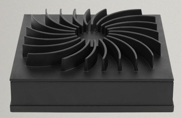
Petite Downlights showcase the patented\* L-Vortex™ heat sink technology, which uses a low profile, spiral fin design to create a vortex of air that effectively prevents the LED from overheating and ensures optimal performance. This design not only enhances the lifespan of the luminaire but also allows for seamless integration into any ceiling type whether IC-rated or non-IC-rated.
