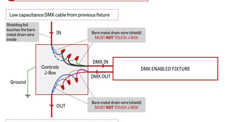
Low capacitance DMX cable to next fixture
