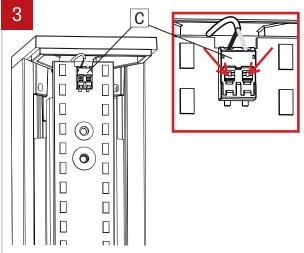
Disconnect LED molex connector (C) by taking a pointed object and pressing on the two tabs on the top.
