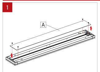
Unscrew and remove the dust cover (A) if provided.
