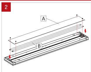
Install the lamps (B) and put back the dust cover (A) back in place.
