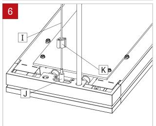
Insert the aircraft cable (I) into the cable gripper (J) and repeat on both sides of fixture. Secure power cord to aircraft cable with plastic clip (K).
