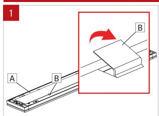
Make sure the power to the fixure (A) is turned off. Unfold the metal clips (B) to get access to the dust cover.
