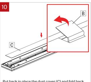
Put back in place the dust cover (C) and fold back the metal clips (B) to maintain the dust cover (C) in place.
