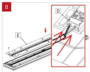
Replace the top reflectors (E) and reconnect the LED connector (D). Screw the top reflector (E) back in place.
