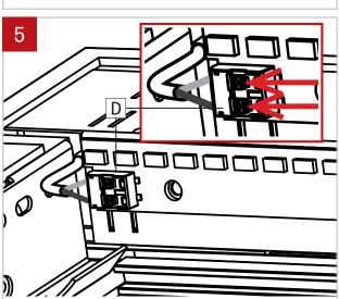
Disconnect LED molex connector (D) on the side reflectors by taking a pointed object and pressing on the two tabs on the top.
