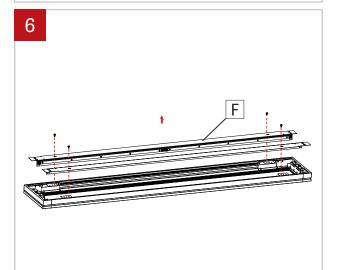
Unscrew the side reflectors (F) and remove them from the fixture.
