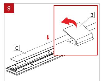
Put back in place the dust cover (C) and fold back the metal clips (B) to maintain the dust cover (C) in place.
