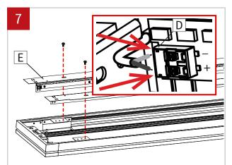
Replace the side reflectors (F) and reconnect the LED connector (D). **NOTE: connect white wire into the negative (-) terminal and the black wire into (+) positive terminal.** Make sure that the wires are not hiding any LED diode. Screw the side reflectors back in place.
