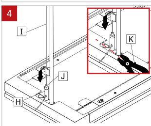
Insert the aircraft cable (I) into the griplock (H). Repeat on both sides of fixture. Adjust the cable (I) length to level fixture by pushing the feeder tube (J). Cut the excess cable with a cable cutter (K).
