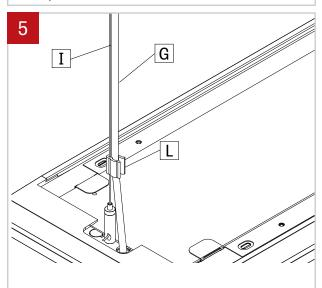
Secure power cord (G) to aircraft cable (I) with plastic clip (L).
