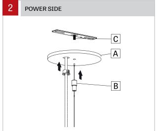
Secure canopy (A) with slip ring (B) on threaded rod (C). For a continuous system, please proceed to step 6.
