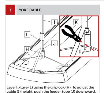
Cut the excess cable with an aircraft cable cutter (K).
