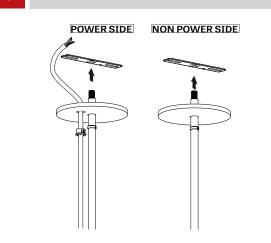
In the case where the luminaire is installed on a grid ceiling, the power cable will pass outside of the stem.
