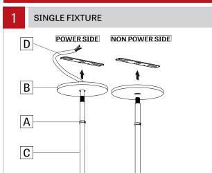
Make sure that the power to the fixture is turned off. Slide the slip ring (A) and the canopy (B) onto the stem (C) and leave some space. Screw the junction box crossbar (D) onto the stem (C).
