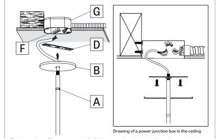
Raise the fixture and tighten the junction box crossbar (D) with screws (by others) to the iunction box (G). Make wire connection with wire connectors (F). Then slide the canopy (B) and thighten the set up with the slip ring (A).
