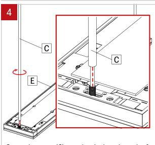
Screw the stems (C) onto the nipple at the ends of the fixture (E).
