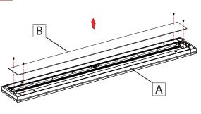
Make sure the power to the fixure (A) is turned off. Unscrew and remove the dust cover (B) (if provided).
