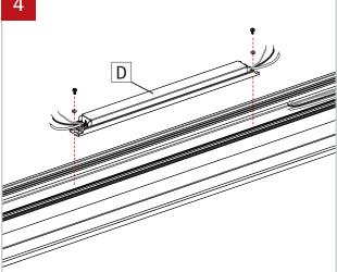
Unscrew the driver (D) from the fixture. Replace
