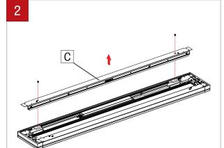
Unscrew the side reflector (C) and remove it.
