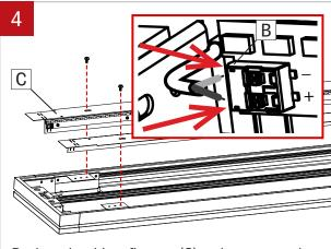
Replace the side reflectors (C) and reconnect the LED connector (B). NOTE: connect white wire into the negative (-) terminal and the black wire into (+) positive terminal. Make sure that the wires are not hiding any LED diode. Screw the side reflectors back in place.
