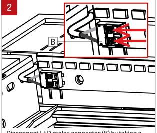
Disconnect LED molex connector (B) by taking a pointed object and pressing on the two tabs on the
