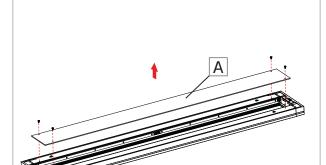
Make sure the power to the fixure is turned off. Unscrew and remove the dust cover (A) (if provided).
